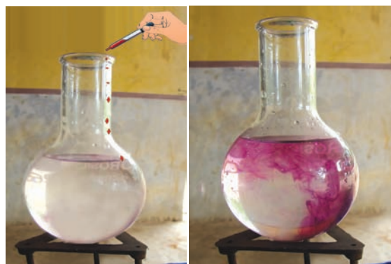
Fig - 6: Diffusion of potassium permanganate in water
