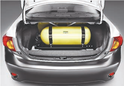
Fig - 2: CNG cylinder in a car
